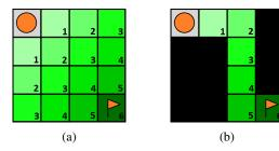
Figure 2: An agent moving on a grid map from a corner to the opposite one. The numbers represent at what timesteps the agent can reach the given vertex.
