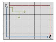
Figure 11: The gradual building of  $SP_i^{Dist}$  from  $s_i$  to  $g_i$  by a greedy approach. The currently build green path has a choice. Moving downward will be chosen since it maximizes the distance to the already chosen paths.
