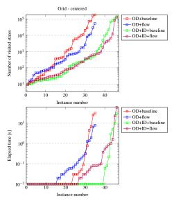
Figure 5: Results of experiments on 7x7 grid with obstacles and clustered starting positions. Top graph shows visited states for ordered instances. Bottom graph shows computational time.
