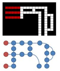
Figure 9: In the top is part of the *Linear* map. On the bottom is its representation as locations that the scheduling model uses. Note that the long sequences of vertices with just two neighbours are abstracted as a single location.
