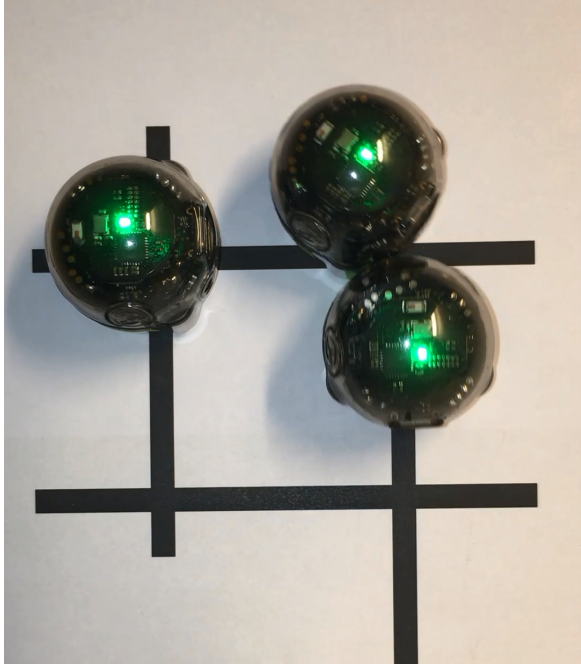
Fig. 14. Example of collision that caused the plan to fail on instance Riddle solved by the model Classic . After the collision, the middle robot was unable to follow the line anymore.
